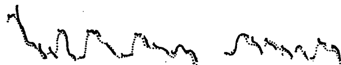
(d) F_0 Variations Due to Phonetic Contents Superimposed on Contours that Incorporate Stress, Constituent Structure, and Sentence Intonation Influences on F_0 Contours.
